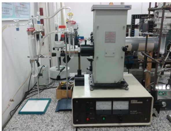
Figure 2.4 Optical configuration for the irradiation in solution.
