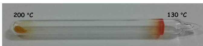
Figure 5.26 Ampoule before crystal growth with temperature of hot and cold ends set.
