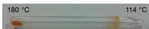
Figure 5.22 Ampoule before crystal growth with temperature of hot and cold ends set.
