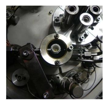
Figure 1.4: top view of the metals evaporation cell.
