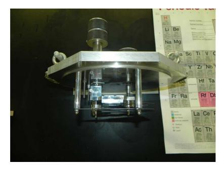
Figure 1.6: chamber lid with as it looks with all the mechanical devices assembled together.
