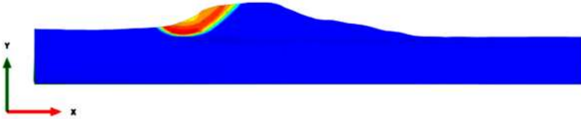
(b) Failure mechanism- Low water level- Factor of Safety: 1.802
