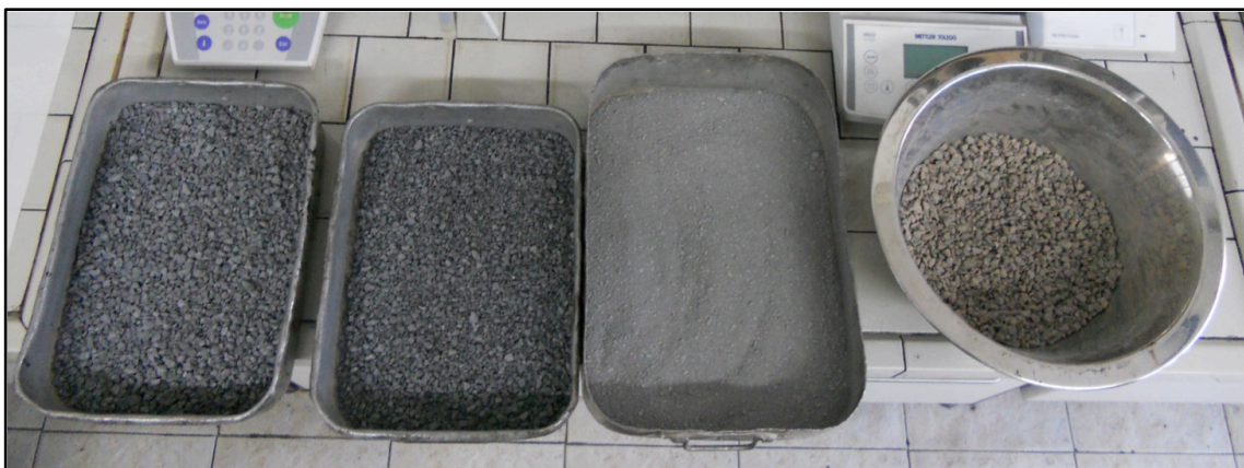
Figure 4.1 Basaltic and porphyritic aggregates used in the mixes for cold-laid multipurpose microsurfacing.
