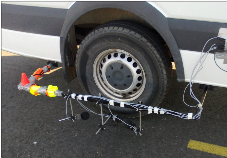
Figure 5.11: Layout of the CPX and OBSI noise testing setup.
