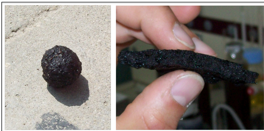
Figure 4.4 Specimen used in the Consistency Test (left) and aggregate covering of a basaltic-mixture specimen (right).
