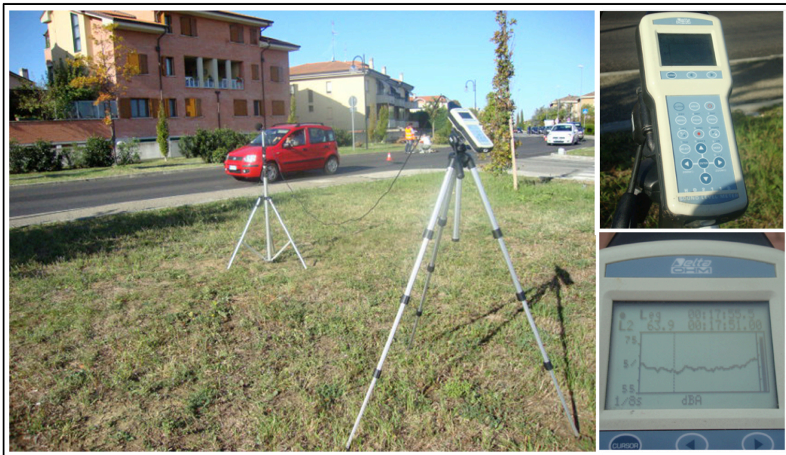
Figure 4.11 SPB noise testing in San Giorgio di Piano (left) with a close-up view of the sound level meter and its display (right).
