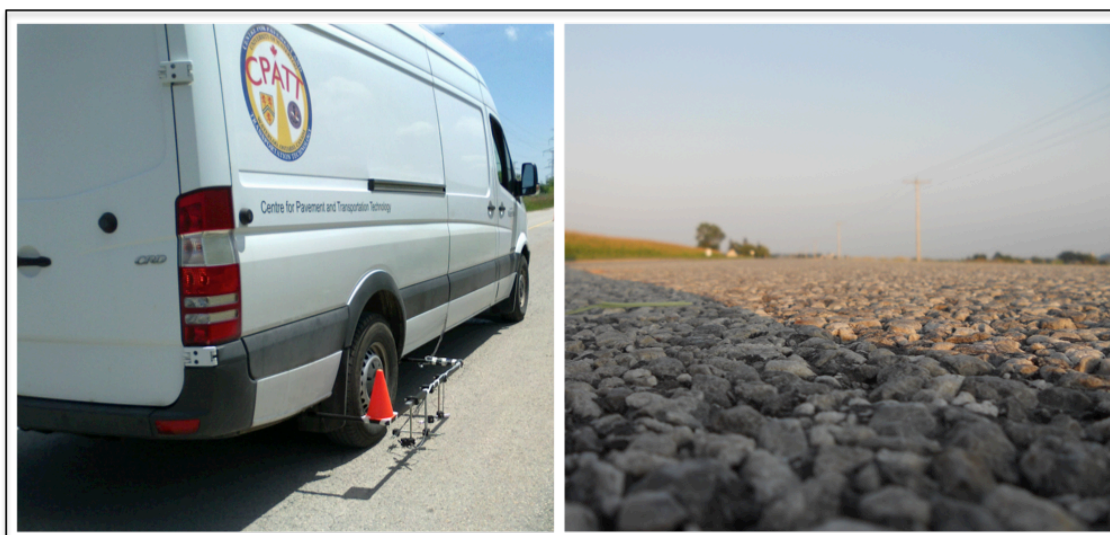
Figure 6.1: CPATT's test vehicle for noise measurements (left) and close-up view of the SMA pavement in Crosshill (right).
