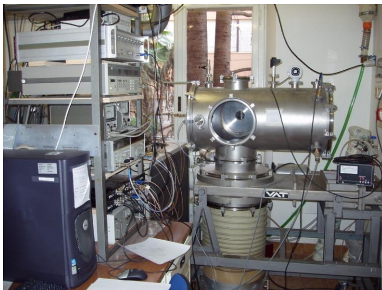
Figure 2.1 Pulsed jet Fourier transform microwave spectrometer built in University of Bologna
