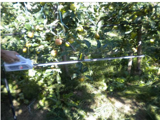
Fig. 6. a) Data collection using the ceptometer (left). b) Black tape used to allowed only 4-5-6 sensors for the readings (right).
