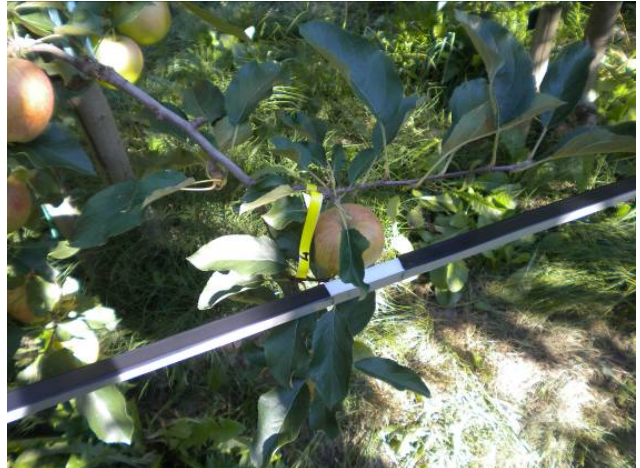
Fig. 6. a) Data collection using the ceptometer (left). b) Black tape used to allowed only 4-5-6 sensors for the readings (right).
