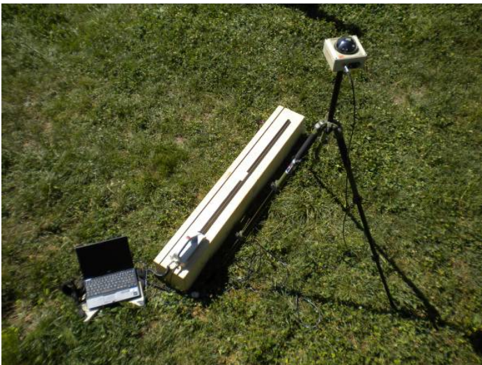
Fig. 5. a) SunScan-SS1 Delta-T Devices Ltd equipped with a sunshine sensor BF3 Delta-T Devices Ltd (left). b) Detail of the Sunshine sensor BF3 (right).
