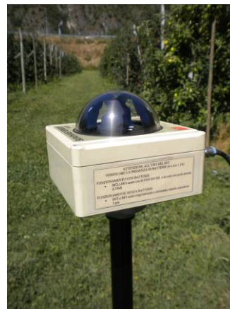
Fig. 5. a) SunScan-SS1 Delta-T Devices Ltd equipped with a sunshine sensor BF3 Delta-T Devices Ltd (left). b) Detail of the Sunshine sensor BF3 (right).
