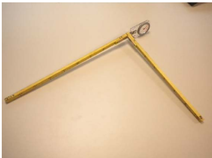
Fig. 1. The woody stick-compass system used to measure the fruit positions. Data were used to draw a 3 dimensional diagram using the two different software (R and Statistica) with an objective to monitor the fruit position and its development on the tree.
