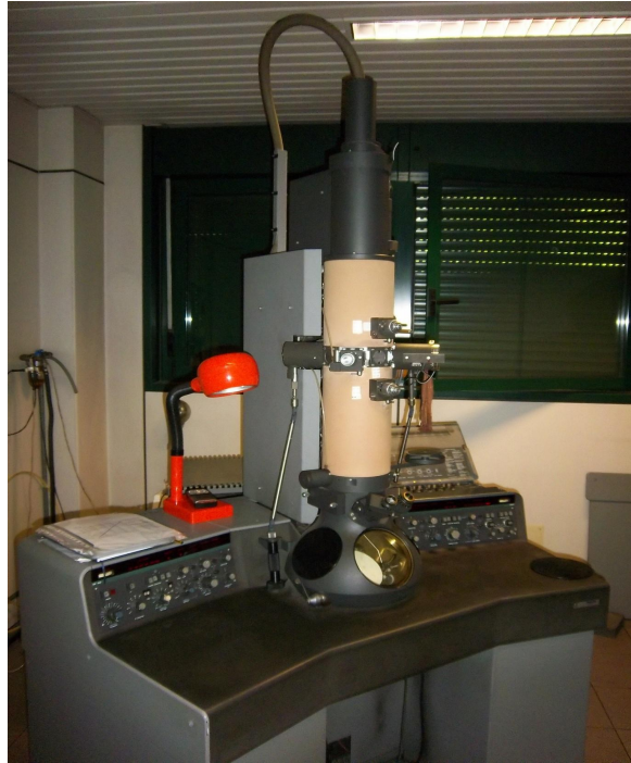
Figure 6.1: The Philips EM440T Transmission Electron Microscope
