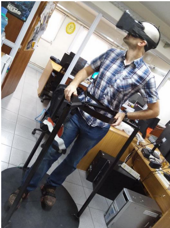
Figure 2: User on the omnidirectional platform. He is wearing a HMD running a Unity3d application on an Android tablet, and the Arduino Uno is attached to his leg.
