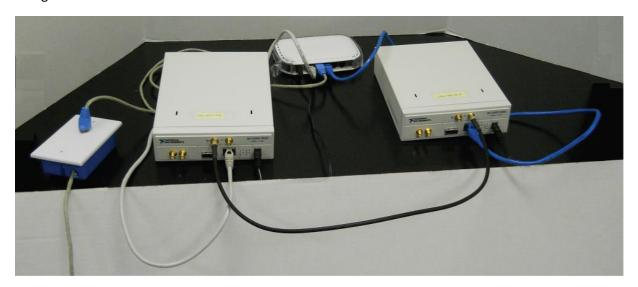
Fig. 8: Loopback Setup Picture
