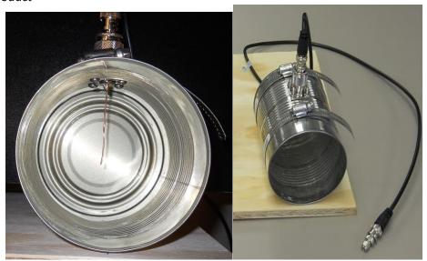
Fig. 225: Assembled Cantenna
