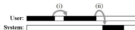
Fig. 1: Turn-taking categories: Black segments represent speech; white segments, silence. (i) Hold transition ( H ); (ii) Switch transition ( S ).
