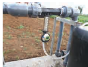
Plate 13 Venturi device as part of a simple volumetric injector used to prepare nutrient solution by diluting stock solutions with water
