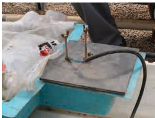
Plate 8 Irrigation of substrate-grown crops: demand tray system located at the end of a tray containing sacks of substrate with a tomato crop (left) and close-up of the demand tray showing the screws controlling the height of two water level sensors (right)
