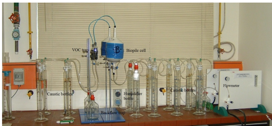
Figure A2. Biopile systems used in this work.
