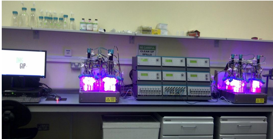
Figure 2: Photo of DASGIP® multi-controlling system photobioreactors for culturing photosynthetic organism.
