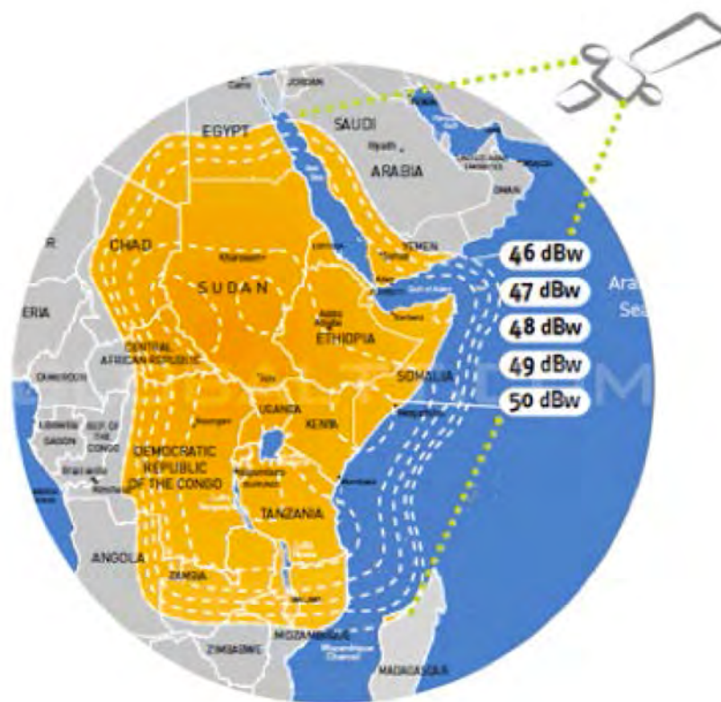
Figure 2: East Africa Ku-band footprint of the NSS-12 satellite, owned by SES (source: http://www.globaltt.com/en/coverage_nss12.html ).
