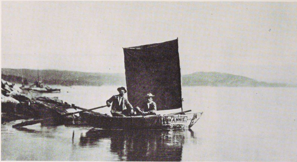
Figure 5 No. 273. THE ANNA (1871), the first boat ever launched upon the lake. Its frame-work was brought up from Fort Ellis and then put together, and covered with tar-soaked canvas. A tent fly made the sail. In it two adventurous members of the survey visited every arm and nook of the lake, and made all the soundings. It is so named in compliment to Miss Anna Dawes, a daughter of the distinguished statesman whose generous sympathy and aid have done so much toward securing these results. 5\frac{1}{2} \times 9 inches. (Caption from 1875 catalog, p. 29. Photo U.S.G.S., Denver, no. 1268.)
