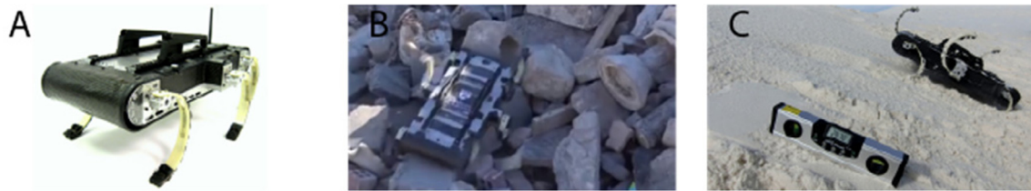
Fig. 3. RHex can traverse a variety of terrains. (A) The XRHex robot. (B) RHex traversing rubble pile. (C) RHex climbing sand inclines.
