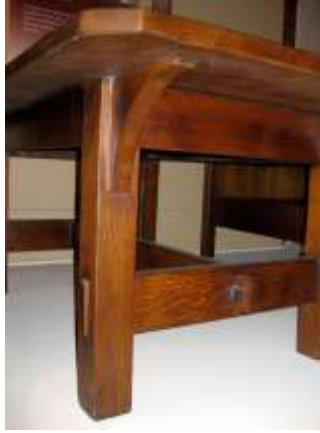
Figure 3.5 Gustav Stickley, Dining Table (1907); photo by author. This is an example of mixed construction. The key locking the stretcher implies that the table can be disassembled. However, the bracket has glued pins, meaning that the bracket would have to be broken off to remove the leg. From the collection of The Stickley Museum, L. & J. G. Stickley, Inc.
