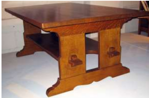
Figure 3.4 L. & J. G. Stickley Co., Library Table (c. 1910); photo by author. This table approximates direct construction. Screws fasten the top to the legs, which Price might criticize, but removing the screws and keys would allow the table to be disassembled and reassembled easily. From the collection of The Stickley Museum, L. & J. G. Stickley, Inc.
