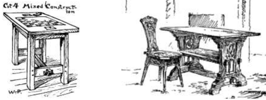
Figure 3.6 William L. Price, Mixed Construction (left) and Direct Construction (right) from The Artsman (1904). Note that in mixed construction on the left, the fasteners at the top of the legs hold the frame together, not the brace with the key.
