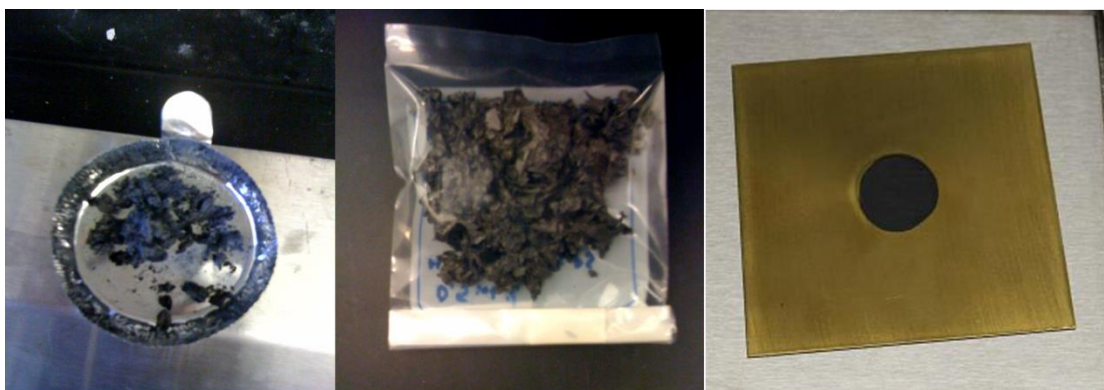
Figure A.3. Resulting composites may look different depending on the wt% of CNTs. After filtering, wet composite are scraped off from the filter (Left). After drying, all composites should look uniform and black (middle). After pressing they should look black and shiny (right).
