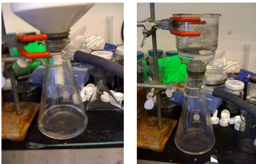
Figure A.1. If using a ceramic porous filter (right, above) no filter paper is needed. If using a normal filter with holes (left, above), choose filter paper that will not dissolve in strong acid. Attach vacuum hose to system. Make sure vacuum is working. Glass ceramic filter is strongly recommended.
