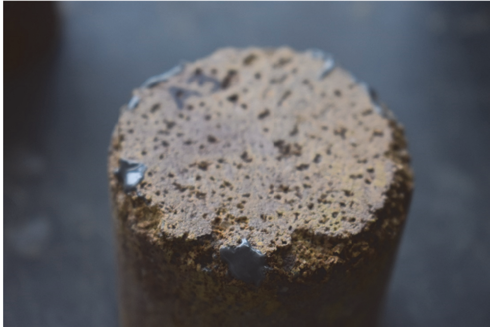
Figure 40: Image of cylindrical sample showing the feathered edge condition. Image Credit: Author
