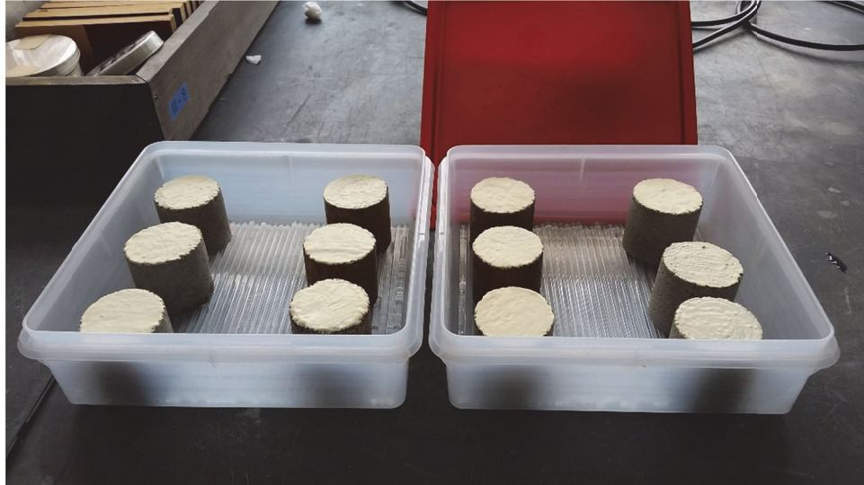
Figure 34: Absorption (immersion) test setup. Image Credit: Author
