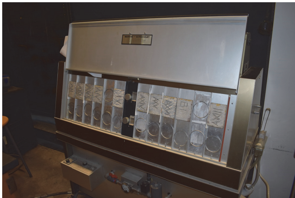
Figure 30: Samples inside of weatherometer. Image Credit: Author
