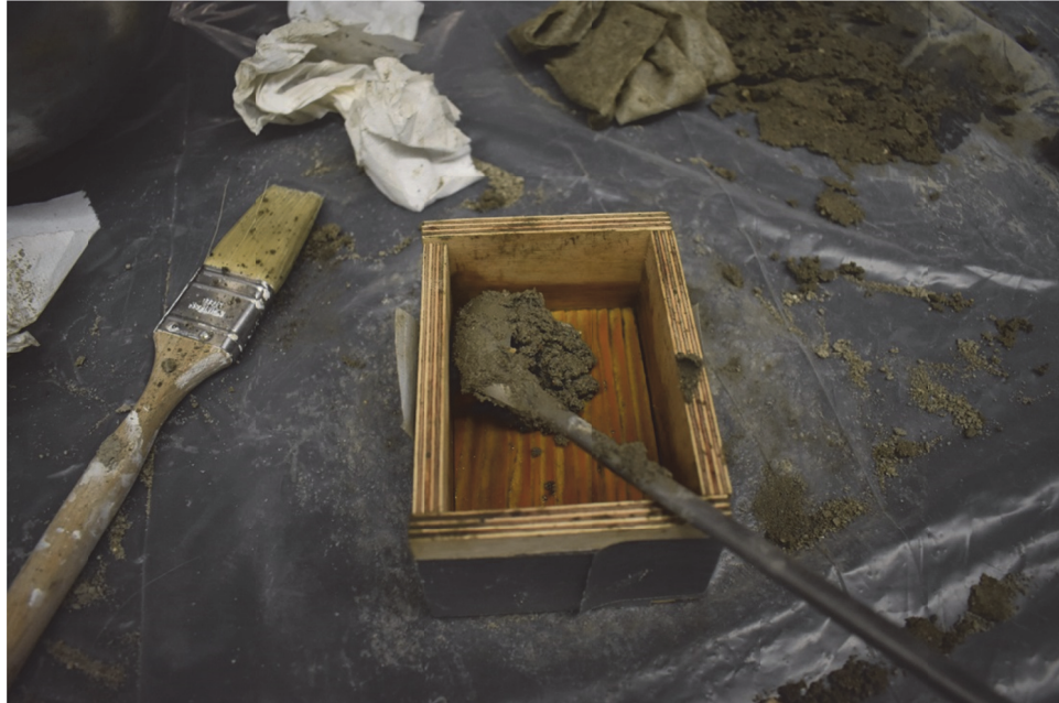
Figure 24: Author Spooning Concrete into Shadowwood Mold. Image Credit: Author
