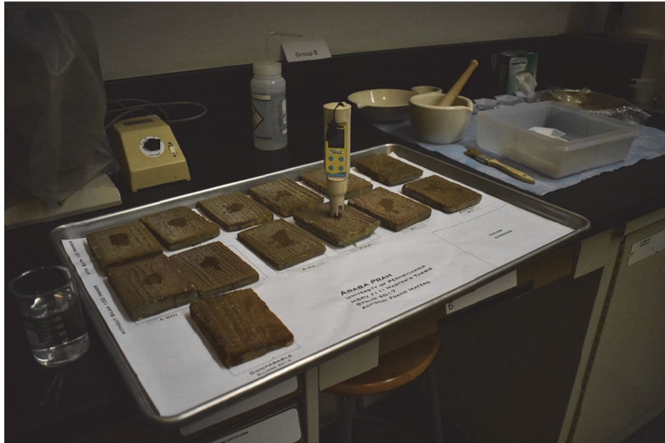
Figure 32: Author taking pH Readings of Accelerated Weathering Cohort. Image Credit: Author
