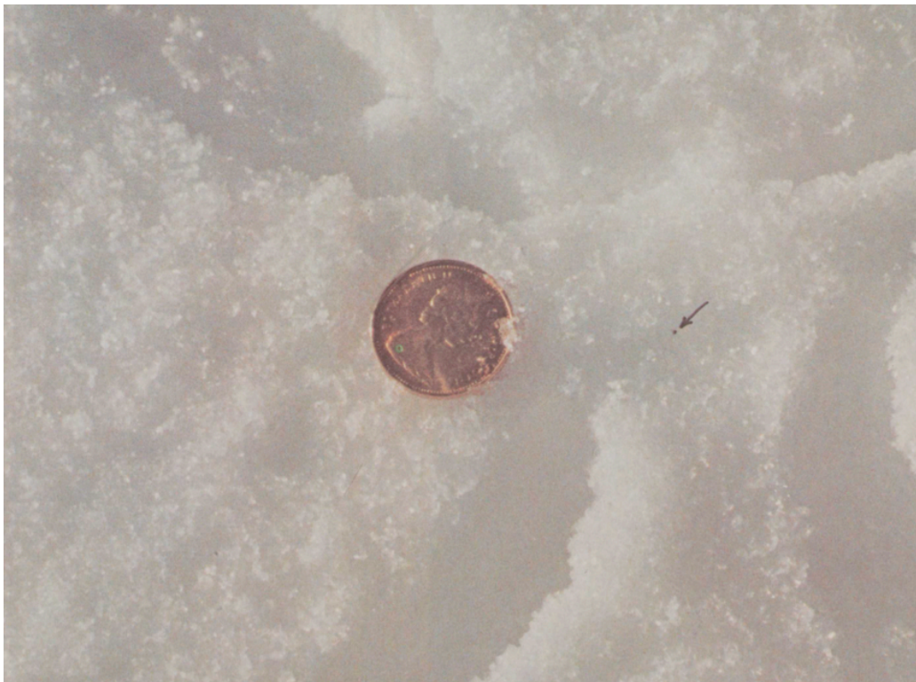
Figure 3.2: A radioactive particle shed during the Kosmos 954 crash, next to a penny for scale.
