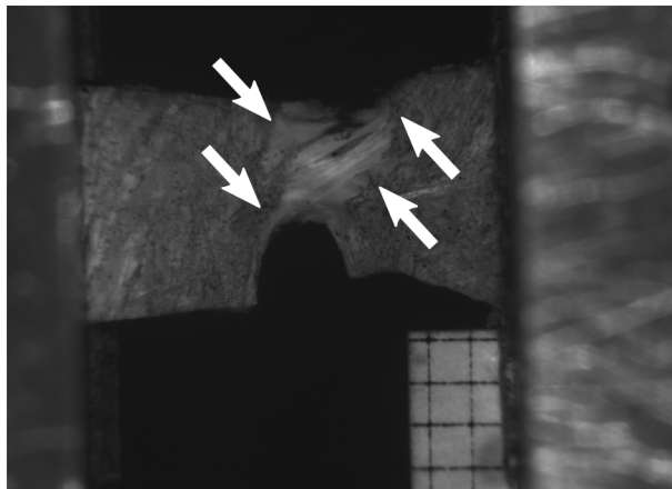
Figure 5.15: Example of rupture (bracketed by arrows) in a radial 90° edge crack specimen by necking and simultaneous rupture across the entire uncracked width. This failure mode is in contrast to crack growth.
