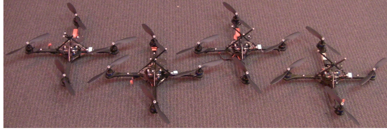
Figure A.1: A team of four Ascending Technologies [5] commercial hummingbird quadrotors used in experimentation.
