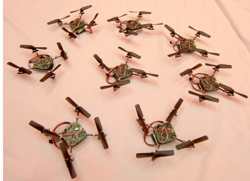
Figure 4.11: Team of eight KMel Robotics NanoQuad quadrotors used in experimentation. More information about these robots is available at www.kmelrobotics.com .
