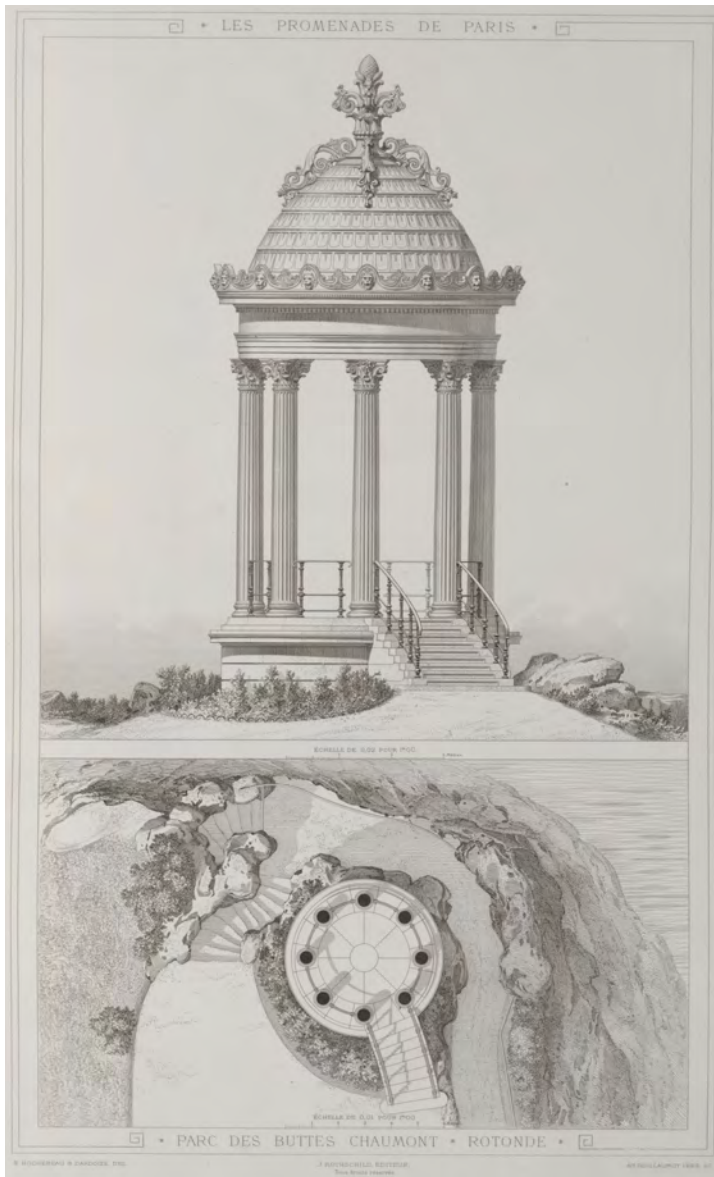
Figure 5.16 Elevation and plan of the rotunda or temple, Parc des Buttes-Chaumont. Designed by Gabriel Davioud. From Alphand, Promenades .
