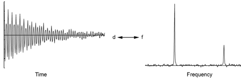
Figure 2.1 An example of spectral estimation is shown for generated data containing two peaks of varying intensity. The time series of an exponentially decaying sinusoid is shown on the left. Only the cosine modulated component is shown for clarity. Application of the Fourier transform to estimate the frequency spectrum produces the spectrum shown on the right.
