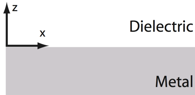
Figure 1.2 | Boundary conditions for derivation of SPPs propagating in the x-direction. The dielectric function varies in the z-direction only. 12 [Adapted from Reference 12]
