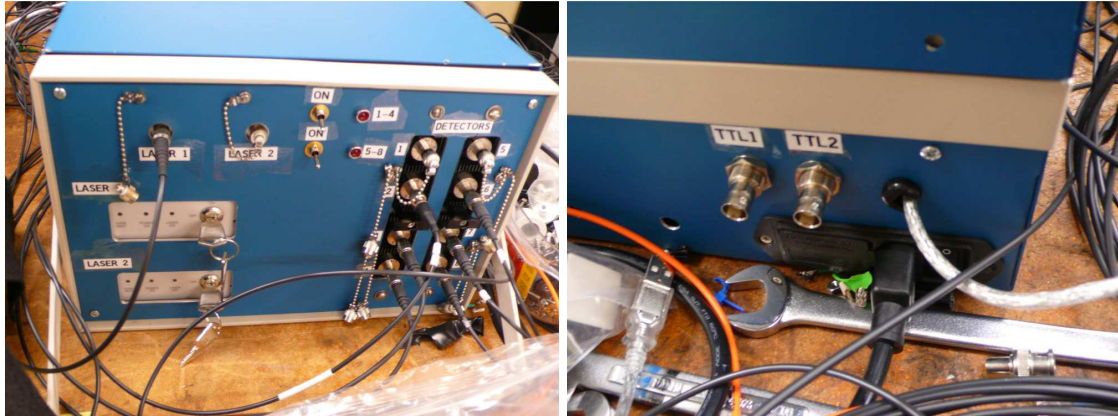
Figure 3.16: Front and back panels of a standard 8-channel DCS module.
