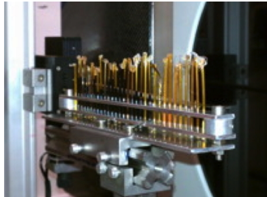
Figure D2. Multi-sample holder designed for rapid acquisition at ESRF ID-15-B.
