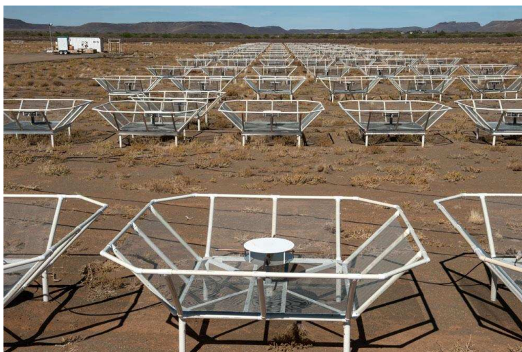
Figure 1.17: A highly-redundant configuration of tiles for the PAPER interferometer, well-suited for power-spectrum measurements. Picture from www.discovermagazine.com
