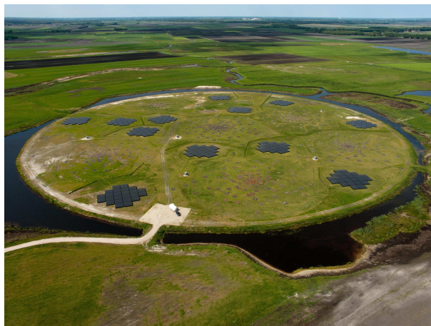
Figure 1.20: The central antenna stations for the LOFAR interferometer. Image taken from www.astron.nl .
