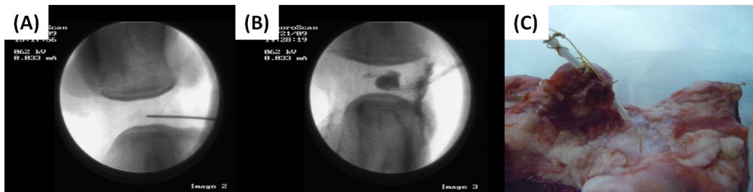
Figure 43: Proof of concept balloon loading placement: (A) Unpressurized placement in center of NP under fluoroscopic guidance, (B) Pressurized balloon, and (C) Securing of balloon.
