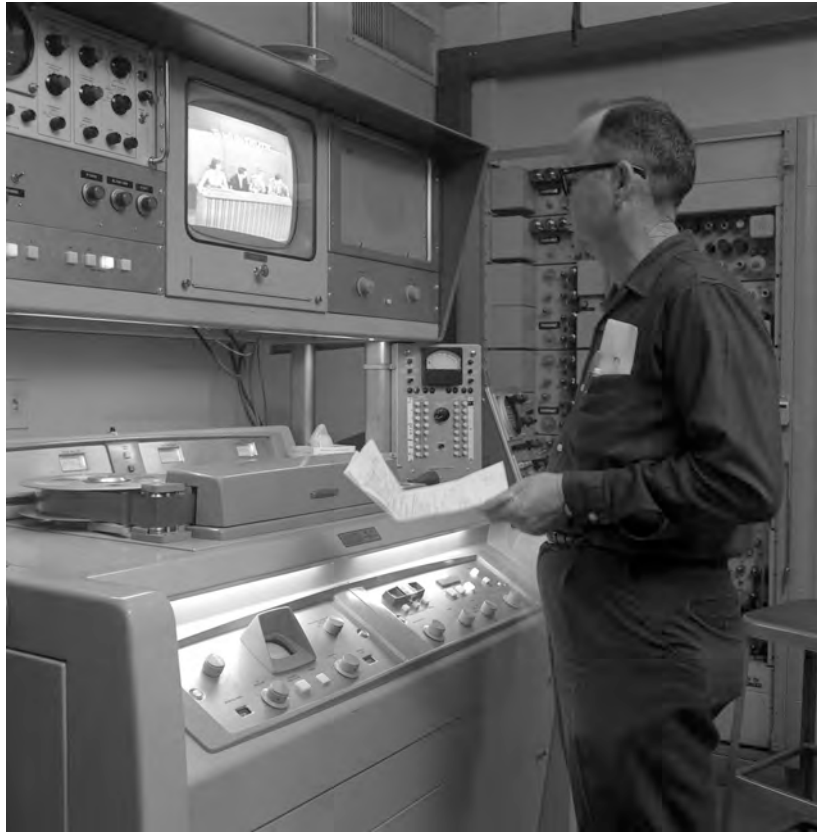
Ampex VR-1000 Videotape Recorder in use at Dallas television station KRLD, c. 1960. 83
