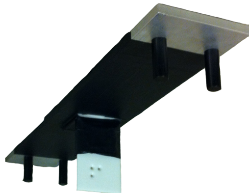
Figure 4.27: Photograph of the profilometry positioning calibration target use to map the images from the profilometry sets and the Gen3 CCD onto the same space. The white plate, with three holes, hangs down in the tank and is used to align the rotational and translational position of the profilometry 3D surface images relative to one another.
