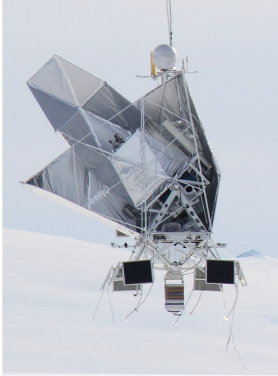
Figure 3.15: Image of BLASTPol in the seconds immediately after launch showing the fully assembled flight configuration of the telescope.
