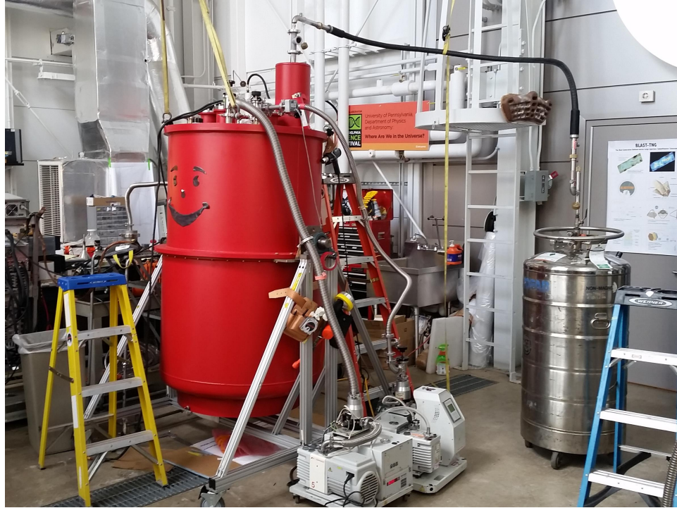
Figure 7.4: An image of the cryostat during the third cooldown showing a liquid Helium transfer in progress as well as two vacuum pumps attached.
