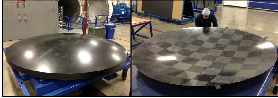
Figure 6.10: Left: The graphite mold that was machined and then hand polished to obtain better than 10\ \mu\text{m} RMS surface accuracy per our optical requirements. Right: The primary mirror at a stage when it was removed from the mold for metrology of the surface. The next steps in its production included attaching the backing structure, plating the surface, and mounting it to the optics bench prior to a delivery in July 2016.
