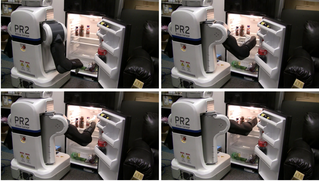
Figure 27: PR2 robot retrieving an object from a fridge using 7D/4D adaptive manipulation planner.
