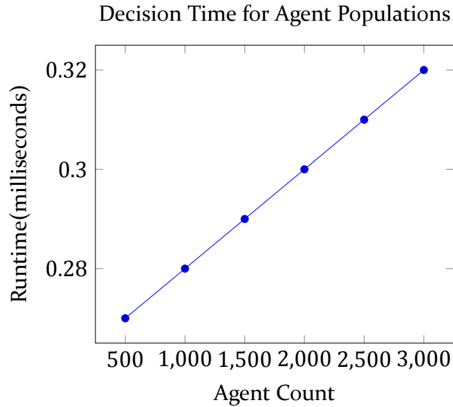
Figure 7.3: The average time taken per-agent to decide their next step action for various population sizes.
