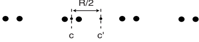
FIG. 5. Two inequivalent inversion centers c and c' in an inversion-symmetric crystal, which differ by half a lattice vector. The parity eigenvalues of Bloch state at momentum k=\pi/R with inversion center chosen at c and c' are different. Crystals terminated at c and c' will have surface charges that differ by an odd integer.
