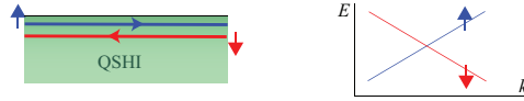
Figure 3.1: Spin polarized helical edge modes of a quantum spin Hall insulator (QSHI).
