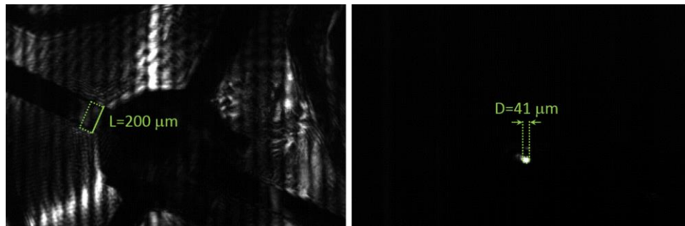
Figure 4-17. The IR images of the device region (left) and laser spot (right) for laser spot size estimation. The images were recorded with the same magnification and pixel configuration. The laser spot size is estimated as \sim 41\mu\text{m} based on the known width (200 \mu\text{m} ) of electrode channel.
