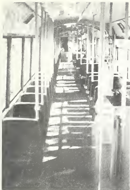
P-13. Interior of a 2.20 m-wide 8-axle double-articulated car (Rotterdam)
