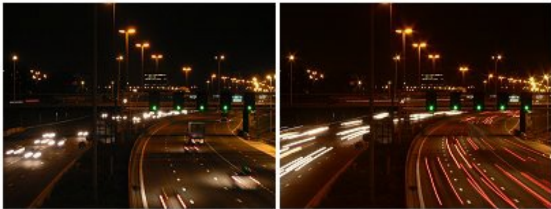
Figure 3.4: Example of high shutter speed necessary to image moving objects. Adapted from (40)
