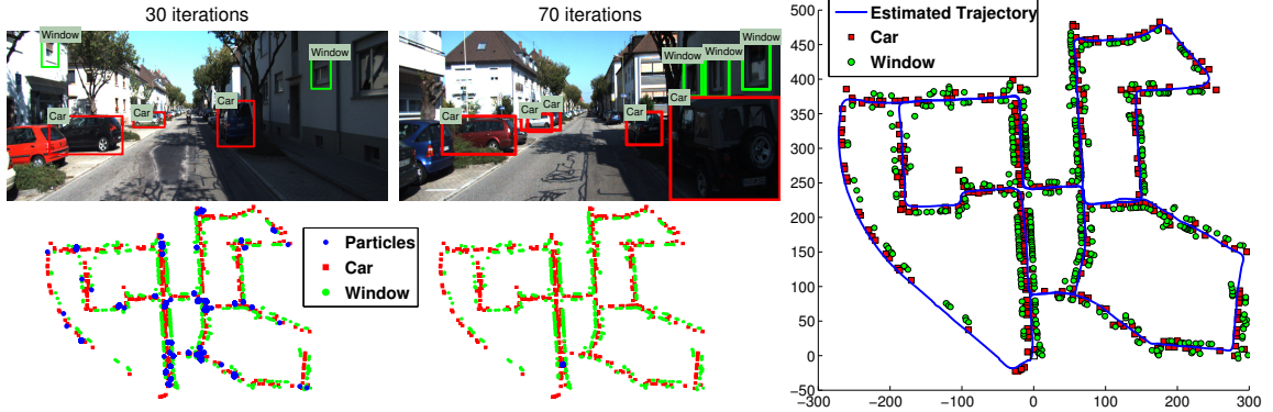
Figure 3.18: Vehicle trajectory estimated via global semantic localization on sequence 00 from the KITTI visual odometry dataset. The left and middle plots show two images with car and window detections and the corresponding particle distributions in the semantic map. The plot on the right shows the semantic map and the trajectory, recovered after unique localization (iteration 70). See Appendix D.16 Extensions 5 and 6 for more details.
