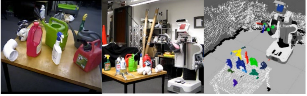
Figure 4.8: An example of the experimental setup (left), which contains two instances of the object of interest (Handlebottle). A PR2 robot with an Asus Xtion RGB-D camera attached to the right wrist (middle) employs the nonmyopic view planning approach for active object classification and pose estimation. In the robot's understanding of the scene (right), the object which is currently under evaluation is colored yellow. Once the system makes a decision about an object, it is colored green if it is of interest, i.e. in \mathcal{I} , and red otherwise. Hypothesis H(0^\circ) (Handlebottle with yaw 0^\circ ) was chosen correctly for the green object. See the video in Appendix D.16 Extension 16 for more details.
