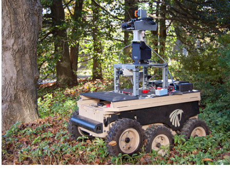
Figure 2.5: The Landshark differential-drive robot (left) tracks a mobile target through a wooded area via range and bearing measurements. The plots on the right show the dependence of the sensor performance on the robot speed, the distance to the target, and the target visibility, which can be obstructed by trees.
