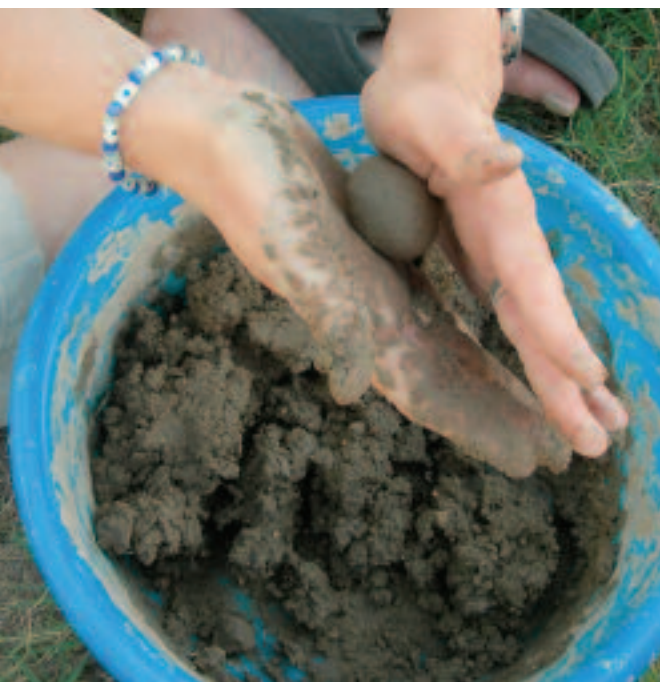
Our mudball mixture consisted of three parts soil and one part clay.
