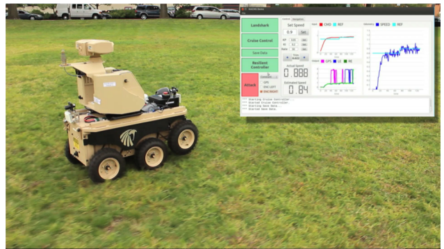
Figure 1: The LandShark vehicle while performing an attack resilient experiment. The user interface on the top right of the figure is used to control the robot, attack sensors, and visualize data.
