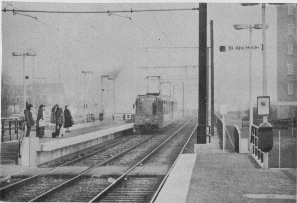
Figure 16. LRT cars in Hannover (W. Germany) serve stations with high- and low-level platforms
