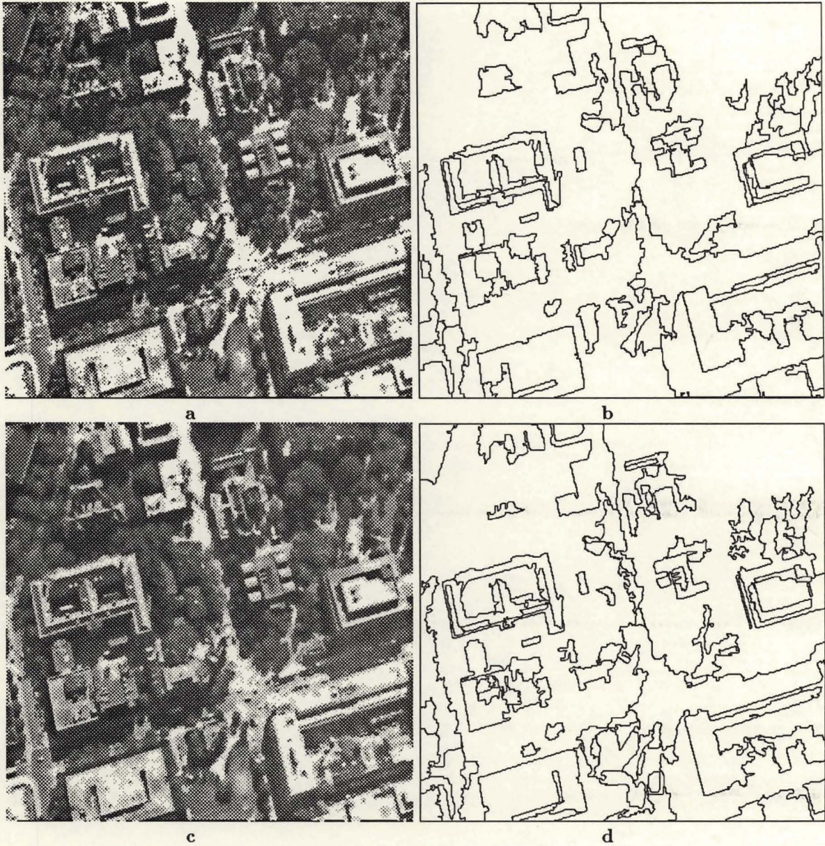
Figure 3: Aerial Photo University of Pennsylvania Campus Original (a), Segmentation (b) Smoothed Original (c), Segmentation of Smoothed Image (d) Though the final segmentations are similar, the internal similarity parameter is automatically set to S = 14 for a to produce b and to S = 5 for the smoother c to produce d.
