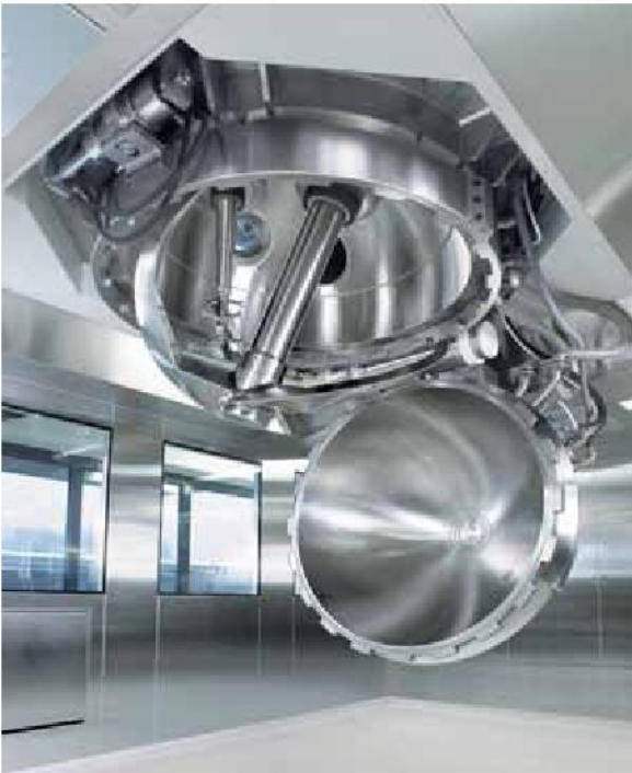
Rosenmund spherical dryer 1000 I
