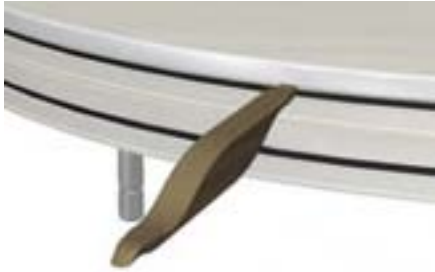
Figure 5.2: Using the removal tool to remove the snap ring.
