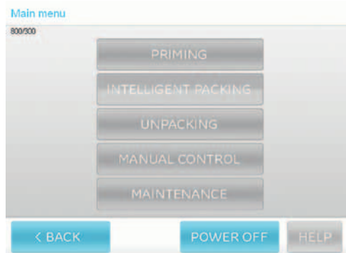
Fig 5. AxiChrom Master controls the packing, unpacking and maintenance of large AxiChrom columns via a touch-screen interface.
