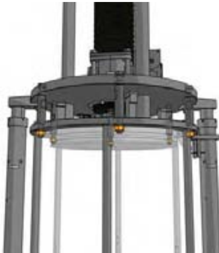
Figure 5.7: Nuts on the top column flange bolts.
