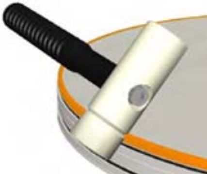
Figure 5.3: Using the groove on the mallet head to lever the snap ring into position.
