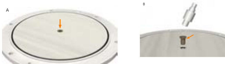
Figure 5.45: A: Media valve is open when the piston is lowered. B: Bed support tool and center bed support screw. Arrow indicates o-ring.
