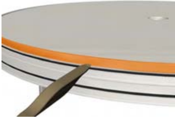
Figure 5.51: Removing the snap ring.
