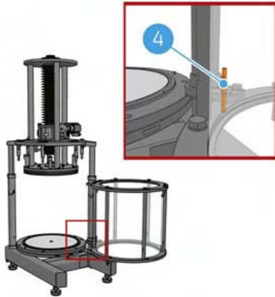
Figure 5.14: Locking pin securing the column tube in the maintenance position.
