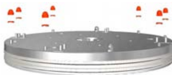
Figure 5.62: Dome nuts holding the bed support and distributor assembly on the backing plate. A: Stainless steel washer. B: Plastic washer.
