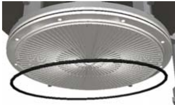
Figure 5.35: Distributor plate o-ring.
