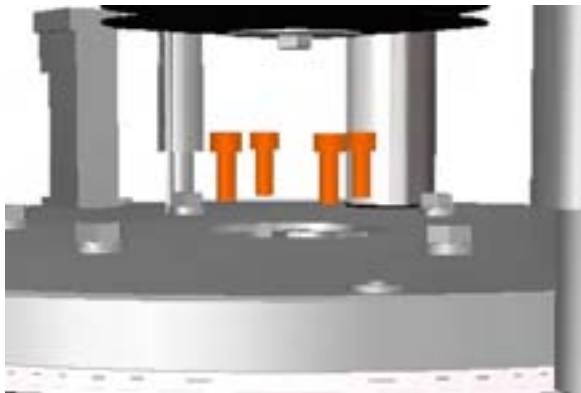
Figure 5.64: Four bolts underneath the inlet/outlet.
