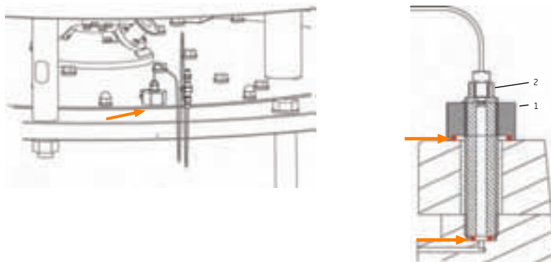
Figure 5.27: Left: Flushing connector. Right: Cross-section showing (1) the flushing connector retaining nut, (2) the flushing connector, and the 2 o-rings indicated by arrows.
