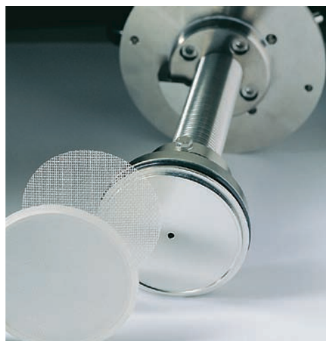
Fig 2. Adapter and net. Flat surfaces give even spread of sample.
