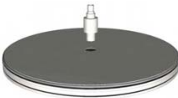
Figure 5.50: Removing the bed support screw.
