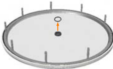
Figure 5.33: O-ring in the center of the bed support.
