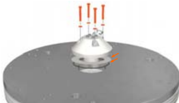
Figure 5.65: Fitting the adapter inlet/outlet. Arrows indicate the plastic spacer and o-ring on 300, 400, 450 and 800 columns.
