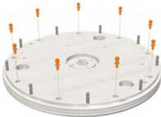
Figure 5.53: Hexagon socket screws holding the distributor ring.
