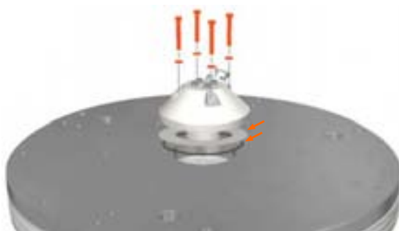
Figure 5.46: Removing the adapter inlet/outlet. Arrows indicate the plastic spacer and o-ring on 300, 400, 450 and 800 columns.
