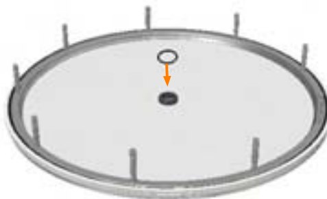
Figure 5.42: Refitting the center o-ring.
