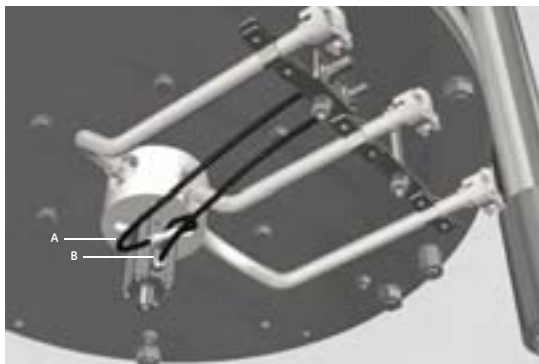
Figure 5.74: Pneumatic tubes A and B , the connection between the pneumatic cylinder and the tube holder.
