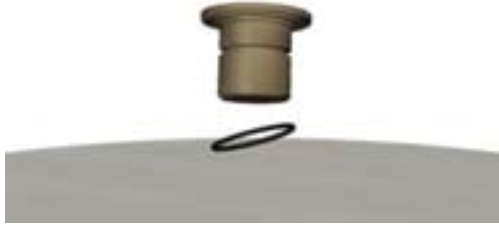
Figure 5.59: Bed support screw and o-ring.
