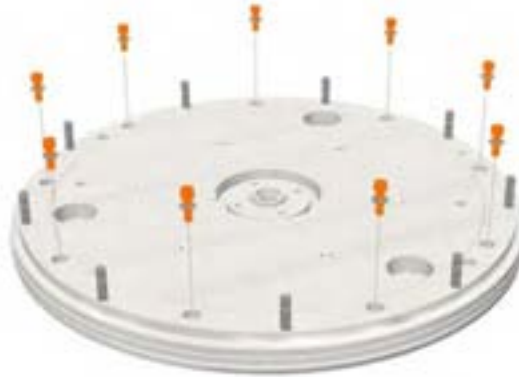
Figure 5.57: Hexagon socket screws holding the distributor ring.
