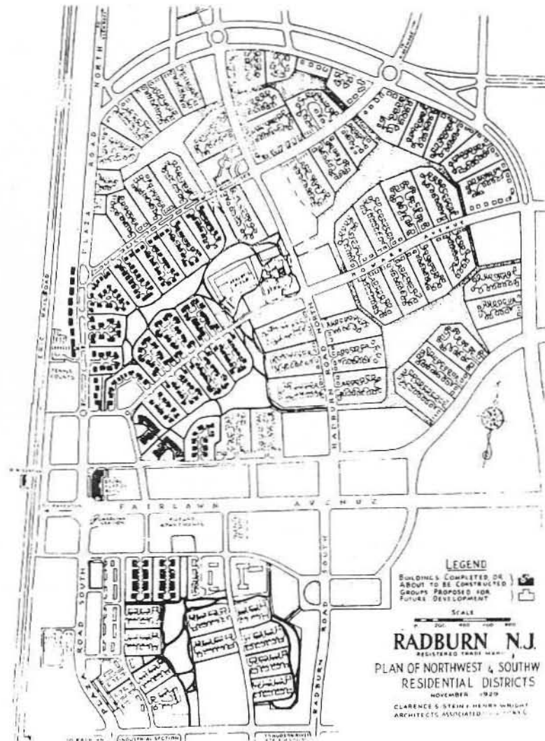
7.1 The final plan for Radburn reveals the hierarchical circulation system and a less rigid land use pattern than preliminary plans.
