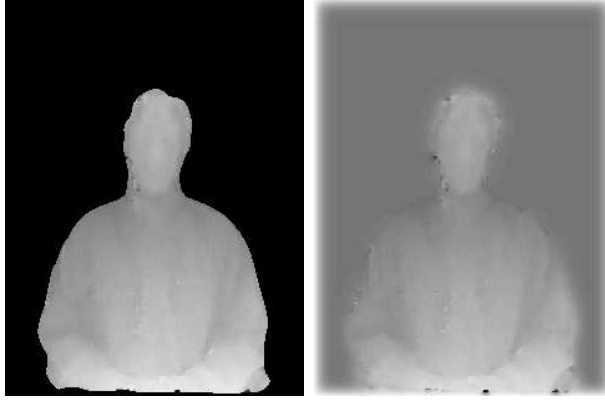
Fig. 5. A disparity map with the background set to a constant value (left) and with a smooth transition to the background. The values within the foreground mask are the same in both cases.
