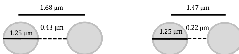
Figure 7: The dotted line indicates the node while the solid line shows the diameter and pitch. The configuration on the right is at the limit of the 110 nm node.
