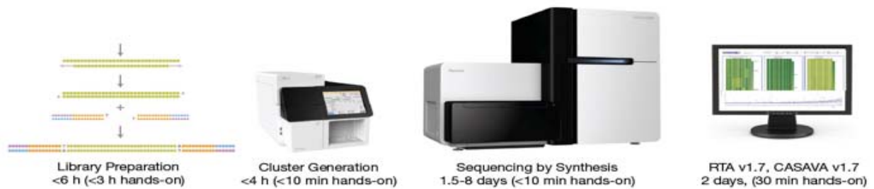
Figure 2.3 Timeline of Illumina’s technology, which demonstrates their throughput deficit. (Image from Illumina, Inc.)
