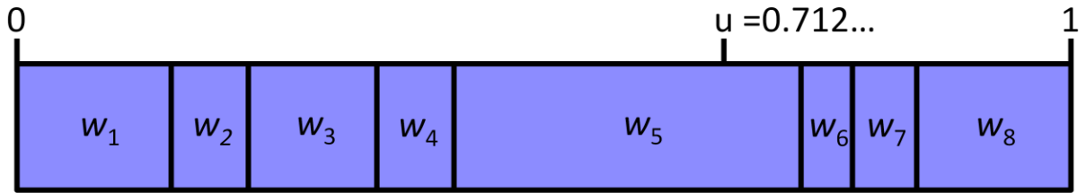
Figure 7 gives an example of how events are selected in a KMC simulation. For every time step, each event is assigned a probability equal to the ratio of its rate to the sum of the rates of all the events for that time step. Each event is given a range on the interval (0,1) corresponding to the probability it will be selected. Then a random number is selected on the interval (0,1) . The event corresponding to the range in which the random number falls is chosen for that time step.
